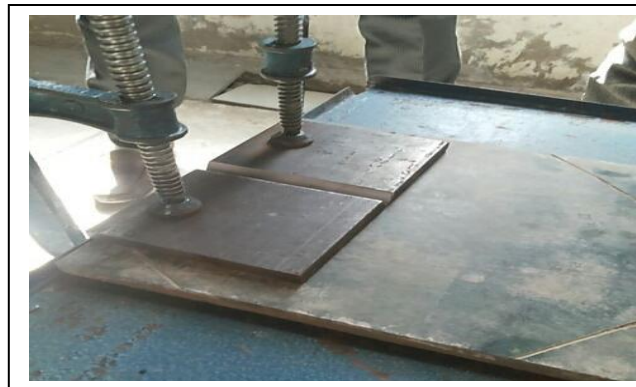
Fig.5: MS Plates clamped on Vibration Table
